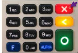
Power up the terminal by plugging in the device or press the red cancel/power
